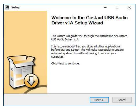
5. When the installer checks the device, if there is a red text prompt: Setup requires that the device is..., please restart the GUSTARD DAC-A22 or re-plug the USB cable.
